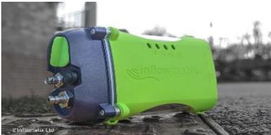
Inflowsys is a high frequency pressure sensor (128 measurements per second) with data logger and integrated communication with the Inflownet platform that allows to identify transient phenomena (water hammer), assess their severity and design mitigation actions.
