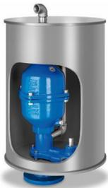
The underground wastewater combination air valve is placed inside a pipe with removable cover, whose base includes an innovative sectioning device. A drainage composed of a 1" pipe stands out, rises vertically and ends with a threaded ball valve. The single chamber design, compact and reliable, can be equipped with the combination version, combination anti-hammer and air vacuum only on request.
