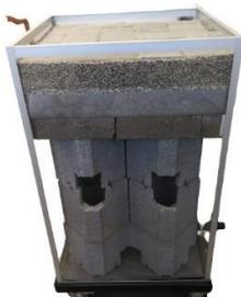
Idrostock is a system consisting of a photocatalytic drainage pavement/soil/gravel base that collects and stores rainwater. This drains to the part below the surface, within a modular system of dry blocks confined within a pre-defined non-permeable space, capable of storing the water it receives.
