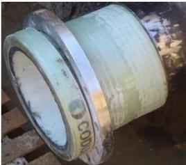
In NoDig systems for pressure pipes, the weakest link is the connection between them. The CODURE flange overcomes this problem by being an innovative solution in the form of a fully anti-slip joint made of glass fibre reinforced polymers with a plug and play installation design. The result is a single, chemically coherent liner-connection entity, that meets the same requirements as the CIPP liner and it is totally independent from the existing pipeline.
