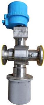
Green Valve System® is a self-sufficient system, capable to regulate the pressure required in a pipeline (like a PRFV valve) and at the same time to measure the flowrate without needing to be powered, using the energy gained from the fluid passing through the valve. Developed in collaboration with the hydraulic division of “Politecnico” university of Milano, it represents a game changer tool for improving the efficiency of water networks.
